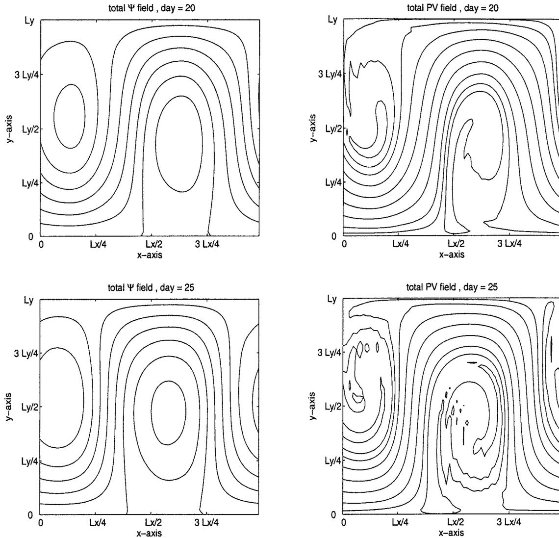
FIG. 7. Snapshots of the streamfunction and potential vorticity evolution for the case  $U_0 = 33 \text{ m s}^{-1}$  and  $h = 400 \text{ m}$ .
