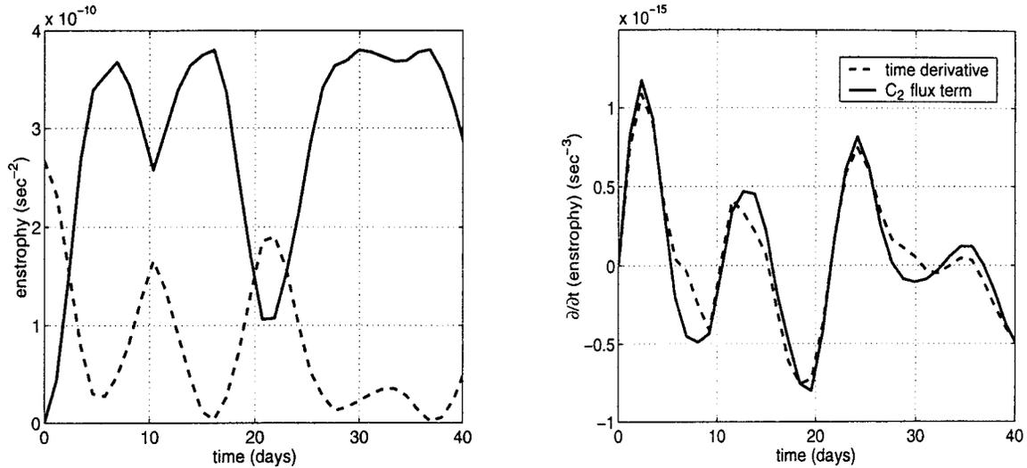
FIG. 6. Left: Time series of wavenumber ( $k, l$ ) enstrophy (solid line) and mean available potential enstrophy (dashed line) for  $U_0 = 46 \text{ m s}^{-1}$  and  $h = 2000 \text{ m}$ . Right: Comparison between time tendency of wavenumber ( $k, l$ ) enstrophy and term  $C_2$ .
