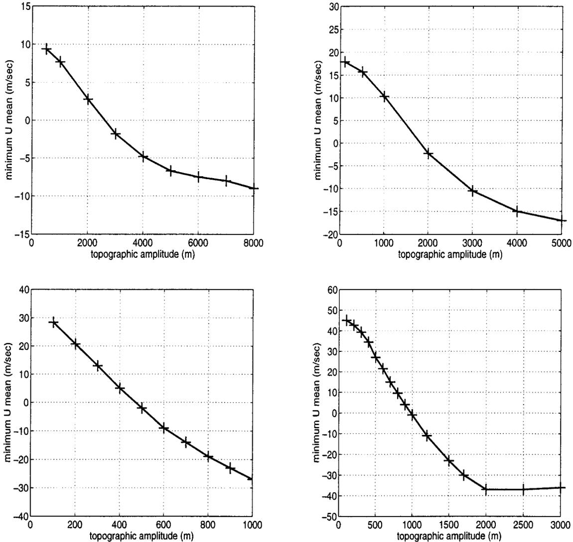
FIG. 5. Minimum zonal mean wind, averaged over the center of the channel, as a function of the topographic forcing. Results for four different basic states:  $U_0 = 10, 18, 33,$  and  $46 \text{ m s}^{-1}$ , going from left to right and from top to bottom.
