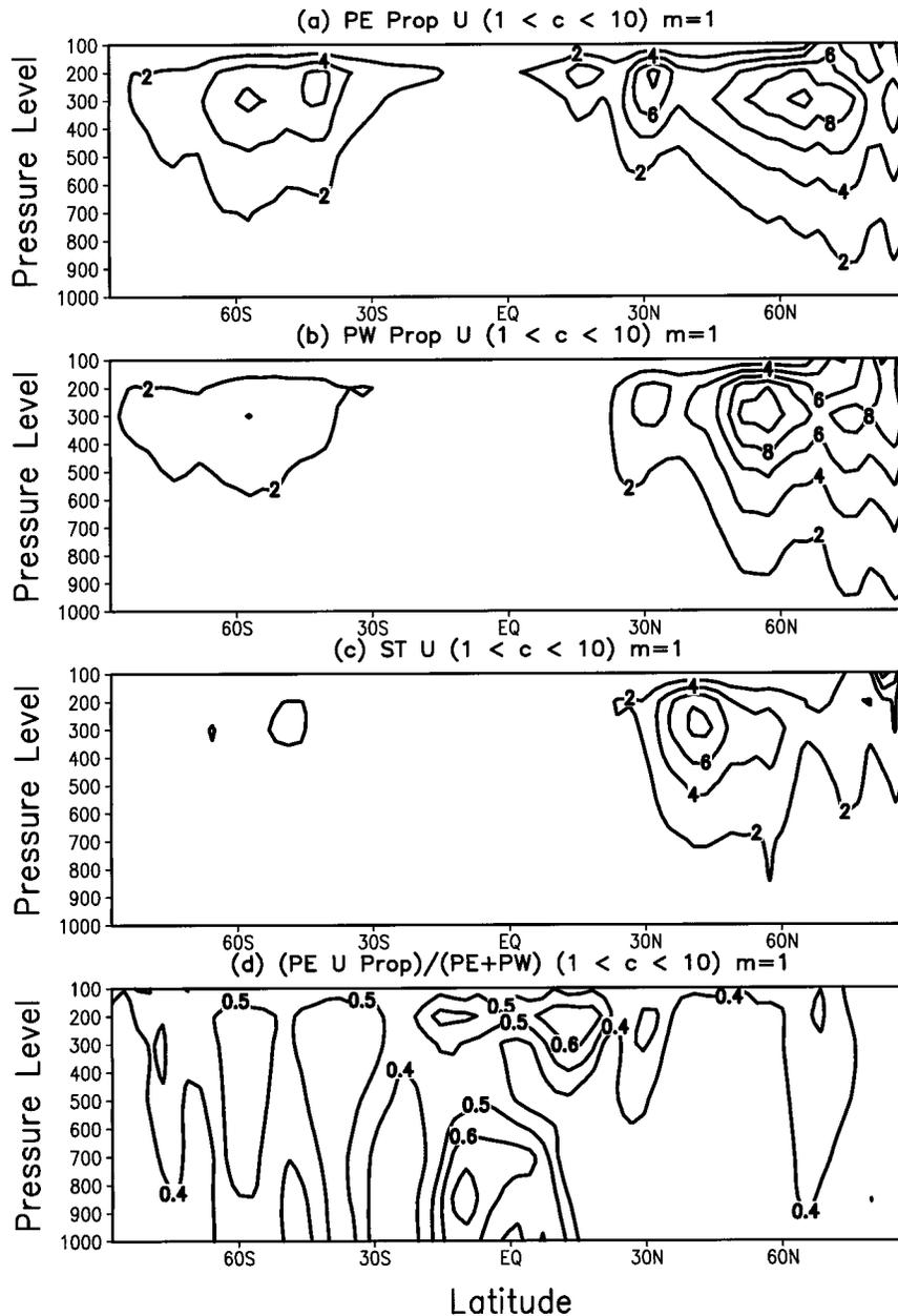
FIG. 3. (a) Eastward propagating wave variance  $PE^*$  for zonal wavenumber  $m = 1$ , summed over frequencies that correspond to phase speeds  $1\text{--}10\text{ m s}^{-1}$ , as a function of latitude and pressure level. (b) Westward propagating wave variance  $PW^*$ . (c) Standing wave variance  $ST$ . (d) Normalized eastward propagating wave variance  $PE^*/(PE + PW)$ .
