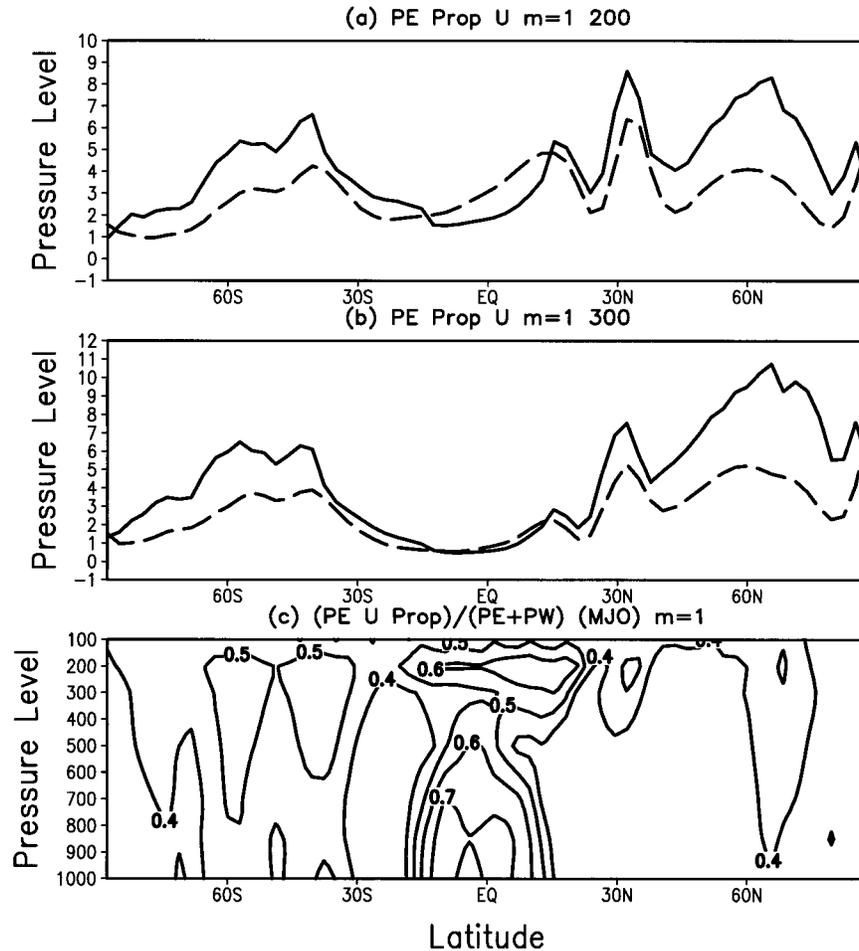
FIG. 5. (a) Eastward propagating wave variance  $PE^*$  at 200 hPa for zonal wavenumber  $m = 1$ , summed over frequencies that correspond to phase speeds  $1\text{--}10\text{ m s}^{-1}$  (solid line), and summed over MJO frequencies (corresponding to periods of 30–60 days, dashed line). (b) Same as in (a) but for 300 hPa. (c) Normalized eastward propagating wave variance,  $PE^*/(PE + PW)$ , where each term is summed over MJO frequencies.
