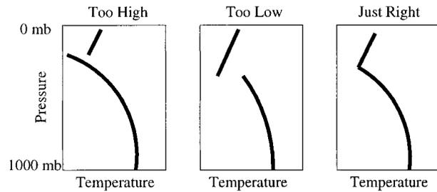
FIG. 5. Schematic depiction of tropopause height determination.
