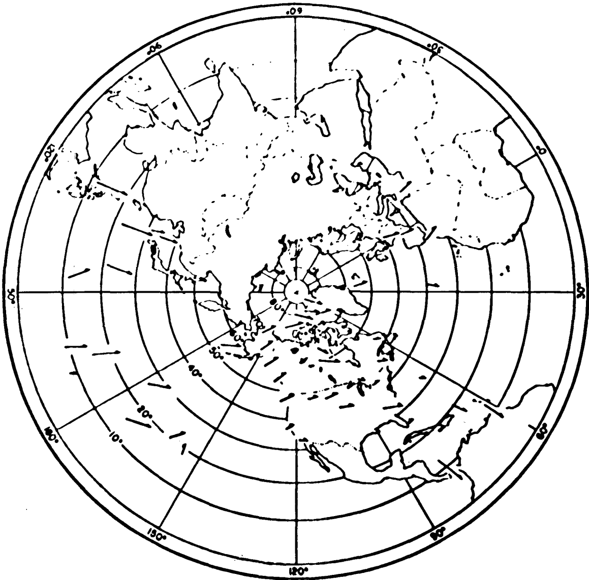
FIG. 14. Annual average wind differences 0000-1200 GMT at 15 mb plotted in vector form (taken from Chapman and Lindzen, 1970). Scale: \frac{1}{4} inch = 2 \text{ m sec}^{-1} .
